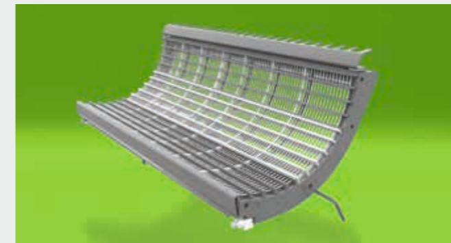
Concave available with different spacing or with the unique segments system.
