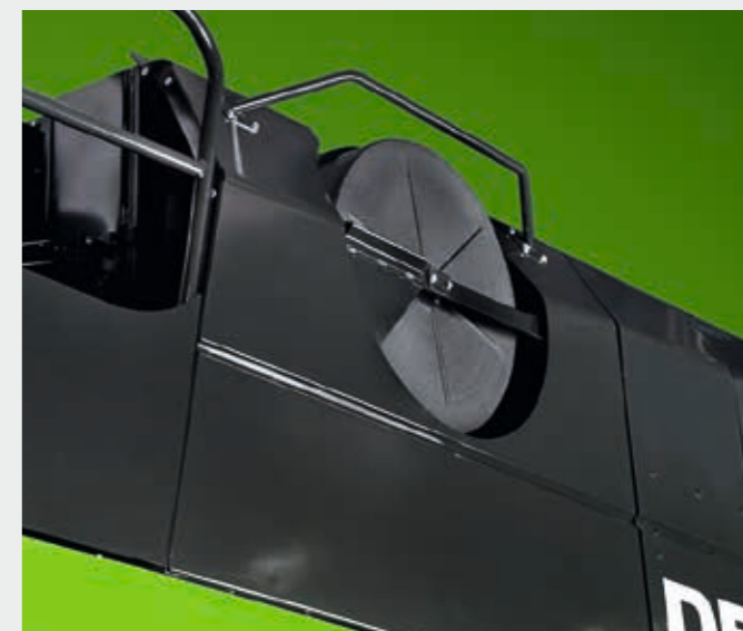
Big rotary screen to ensure maximum efficiency of the cooling system.
