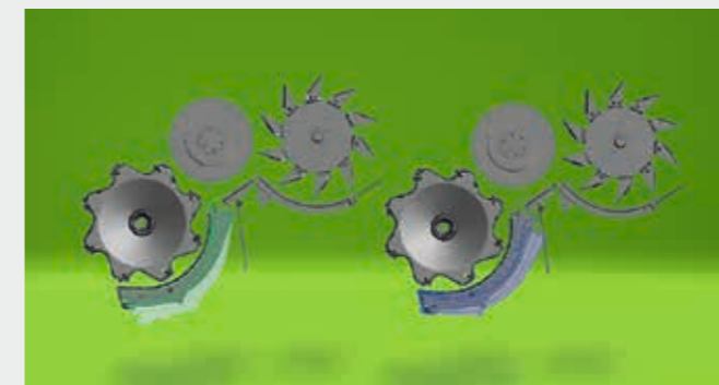
Concave adjustment independently in the front and rear.
