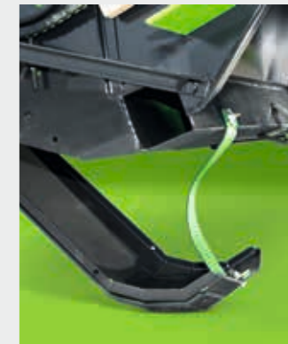
Reliable and robust sensors skids for the Autocontrol system.
