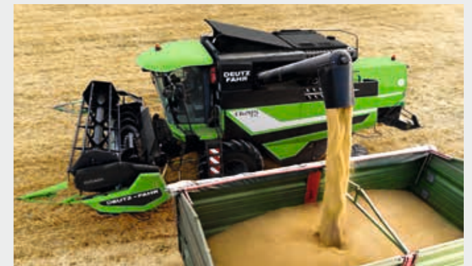
Unloading tube to discharge the grain while working in any position to tall trailer.
