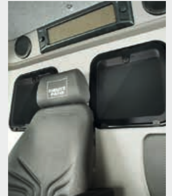
Double grain tank inspection window.
