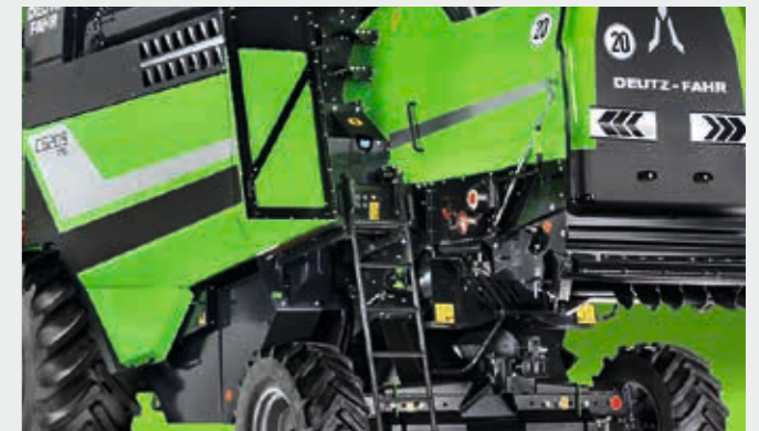
Easy access to the upper part of the combine as well as to refill Diesel and AdBlue.
